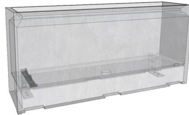
DETAILED AND TRANSPARENT VIEWS OF A SMALL BRACKET FIXING DESIGN THAT INCLUDES LIFTING LUGS
