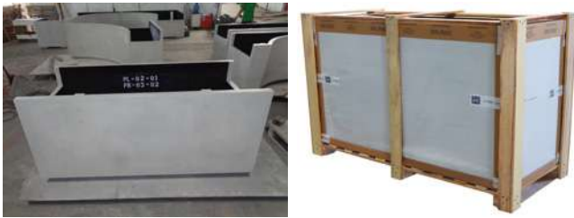
One of the GRC elements during the manufacturing stage and after packing
